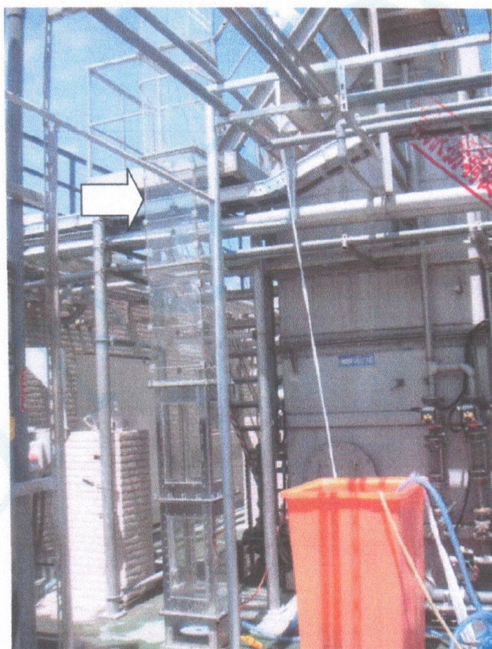
Photo 1. The in-situ testing installation for the measurement of oxygen transfer
